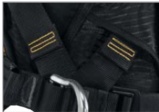
Fall indicators on the sternal and dorsal attachment points. If a fall indicator is visible after a fall, the harness must be retired.
